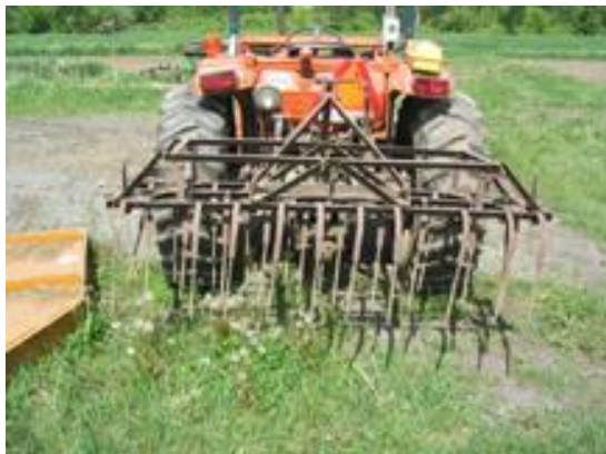
This old Ferguson tine weeder is used for stale bedding fields prior to planting and for blind cultivation over crops like corn while they are still small.
