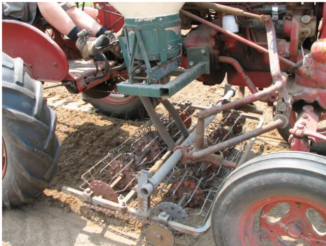
Buddingh baskets belly mounted on an old IH 140 tractor are used to incorporate pre-plant fertilizer into beds and for stale seedbed control of small weeds before planting crops.
