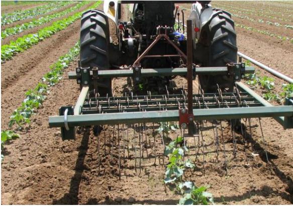
Williams cultivator with tines over the entire bed and C shanks with sweeps in tire tracks.
