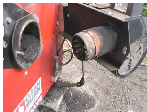
The nozzle and fan inside the burner tend to gunk up and must be cleaned regularly.
