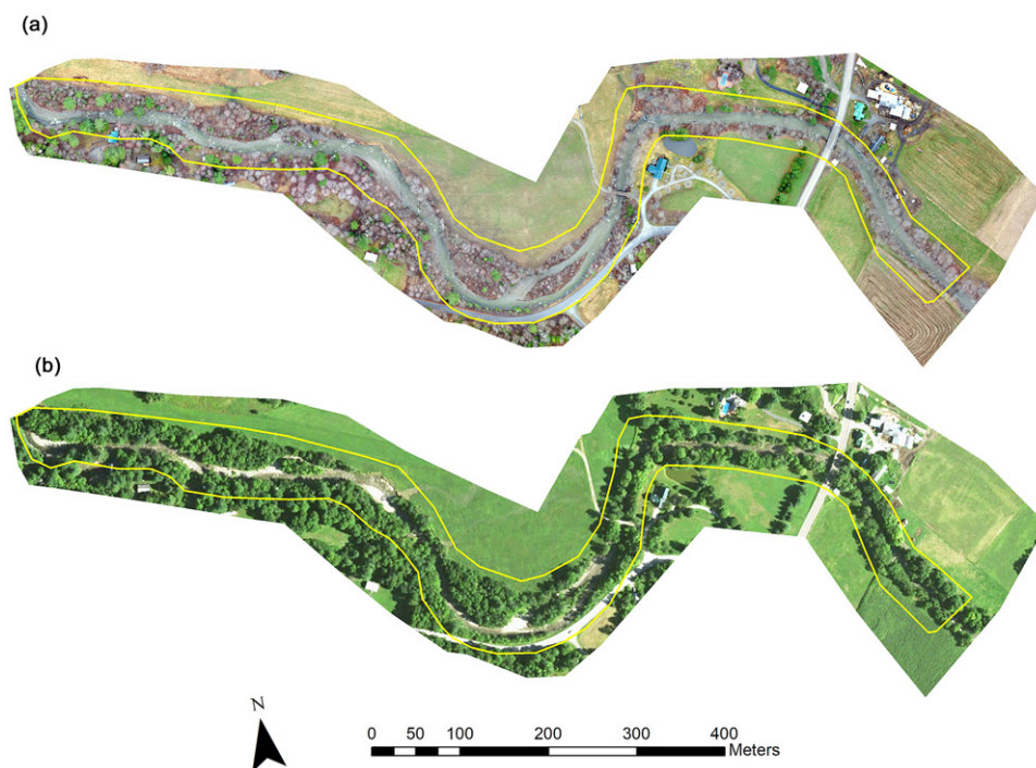
Figure 8. Section of the Shepard Brook as seen in (a) UAS orthomosaic imagery from April 2017 and (b) aerial imagery from July 2016. Area indicated by yellow boundary represents area of river corridor used in the analysis of DEMs. Source: Author
