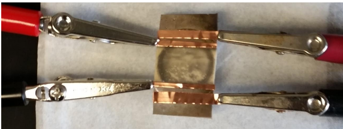
Figure 2: Four-wire setup for electrical testing
