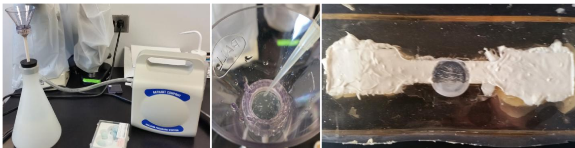
Figure 1: Vacuum filtration setup (left). Using pipette to pour nanowire ethanol solution on filter (middle). Liquid latex mold with nanowires on filter face down (right). These show the simplicity of the nanowire transfer process for the liquid polymers
