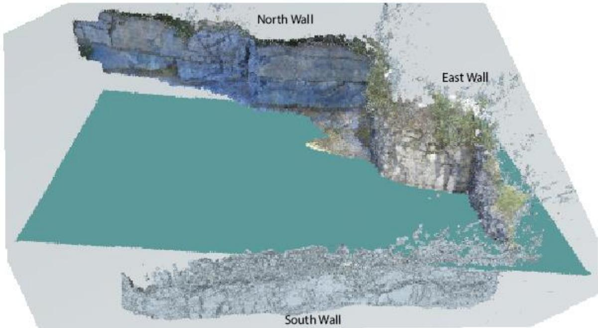
(b) Projection of the ground surface from the top of the South Wall underneath the North Wall, showing the gap where data is not observable from the North or South Walls, but can be seen on the East Wall
