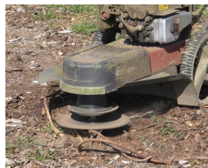
Figure 1. DR trimmer fitted with a modified metal blade for hop crowning.
