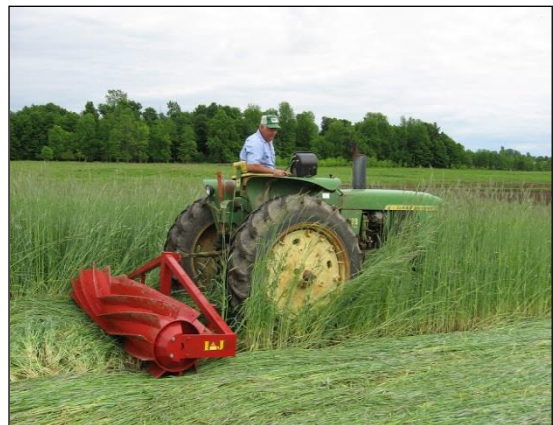
Figure 1. Roger Rainville uses a roller-crimper to terminate a winter rye cover crop.
