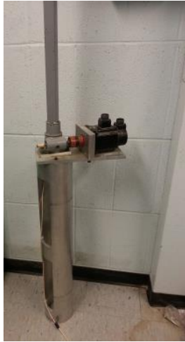
(a) Cone penetrometer
