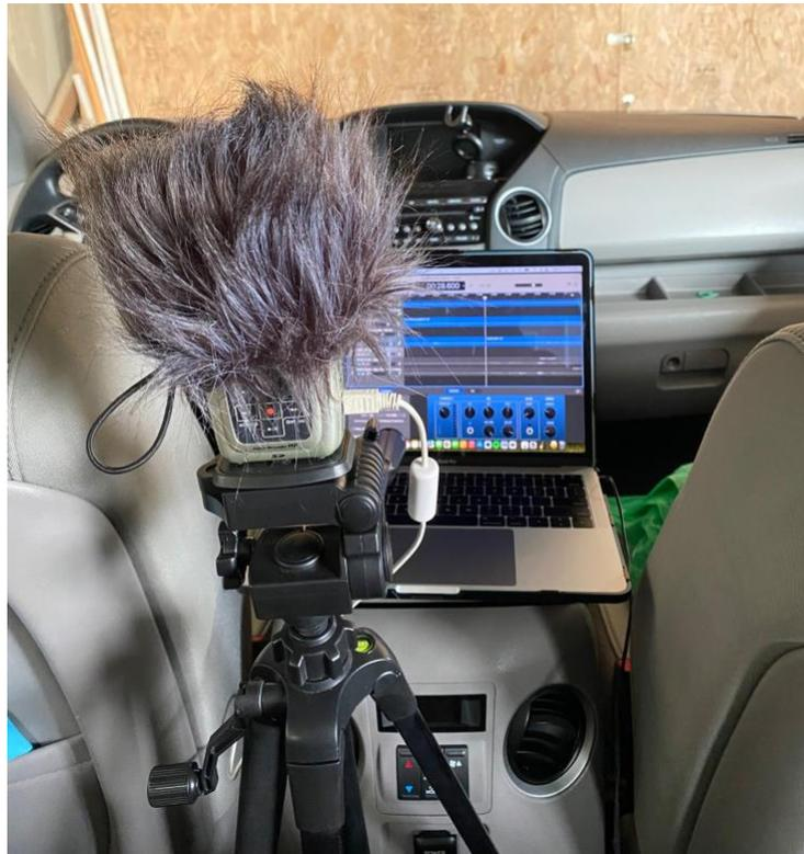
**Figure 5.** The recording setup in a parked car featuring the Zoom recorder on the tripod, with the Garageband display on the computer.
