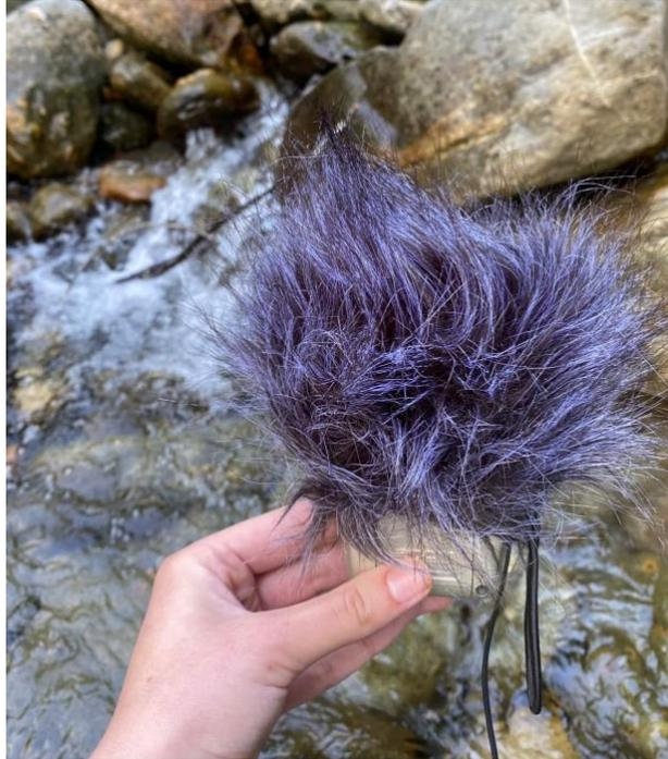
**Figure 4.** The microphone windscreen used when recording.
