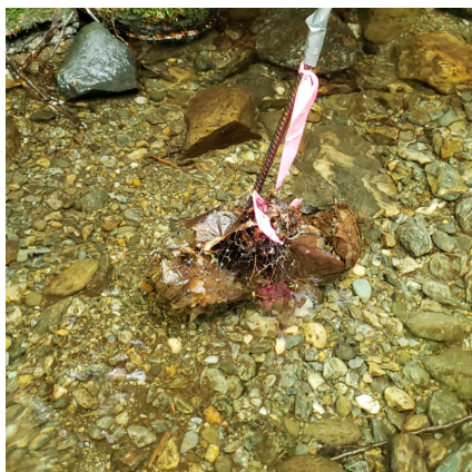
Figure 4: Two leaf bags attached to a piece of rebar in a pool of one of the forested streams (Stevensville Brook).
