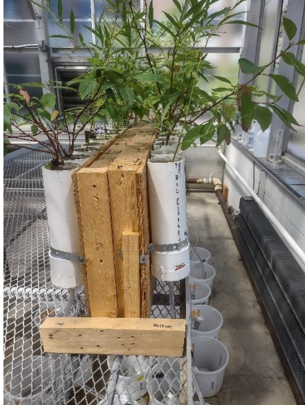
Figure 2. Mesocosm set up; 15 on each side. Buckets below catch leachate.
