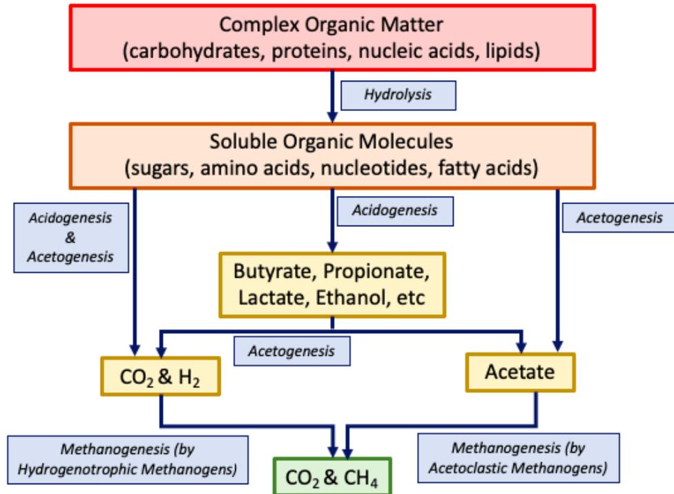
**Figure 1.1.** Anaerobic Digestion Process Diagram
