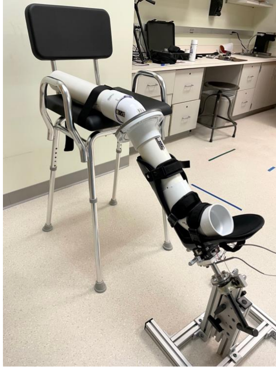
Figure 2: PVC pipe validation jig in the rotational laxity device.
