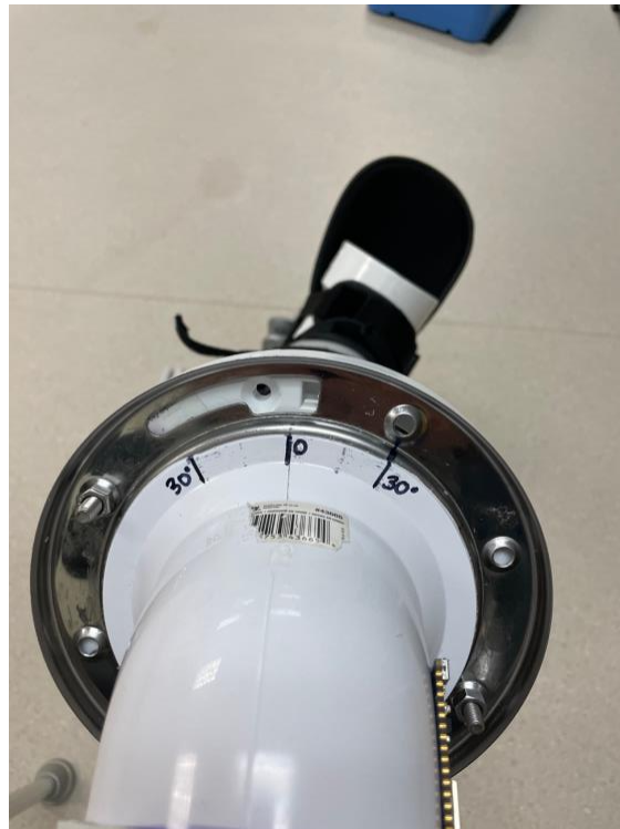
Figure 2: PVC pipe validation jig in the rotational laxity device.
