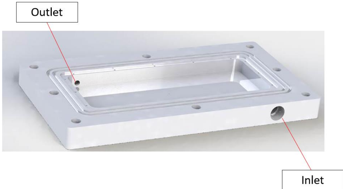
Figure 4: Side view of filtration cell produced for study, showing location of inlet and outlet ports.
