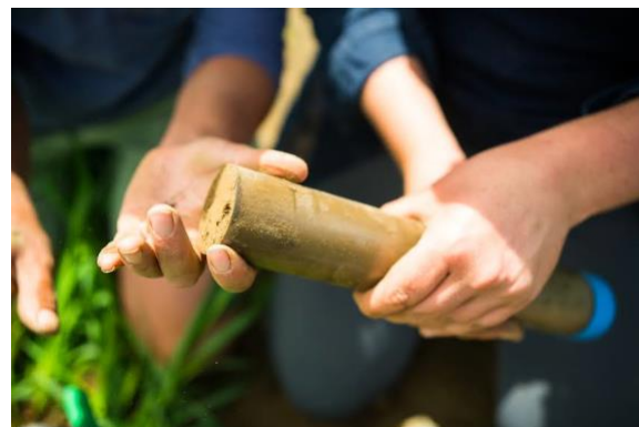
Figure 3. Bulk density soil cores collected for the State of Soil Health project.
