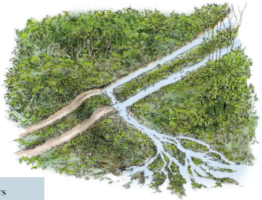
Water bars divert runoff from road and trail surfaces into areas where water can spread and sink into the soil.
