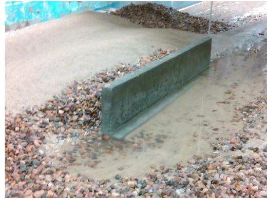
(b) Abutment with erodible approach
