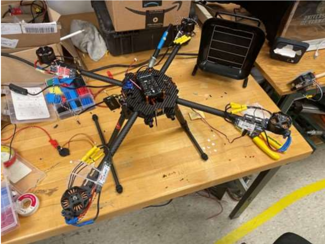
Figure 4. Three-phase AC motors at the end of each arm
