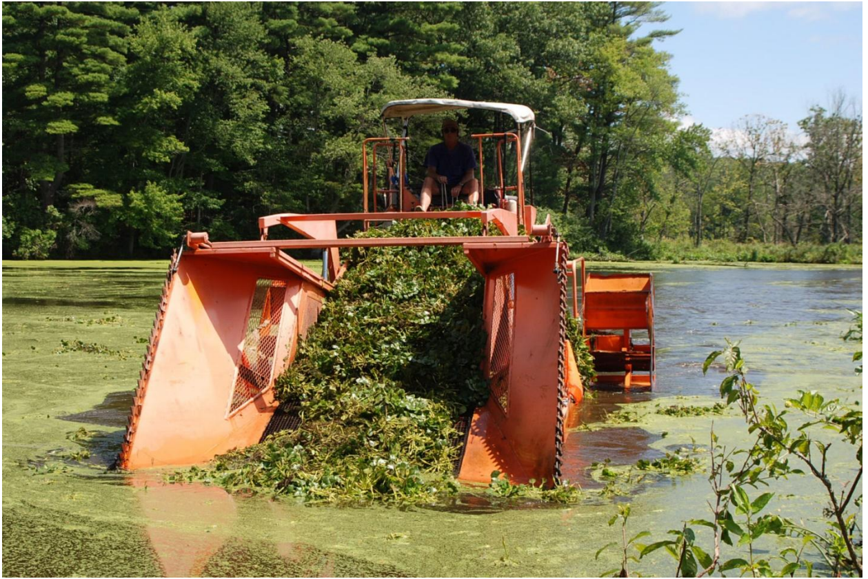
Figure 2-1. Aquatic invasive species mechanical harvester in operation taken by Solitude Lake Management. Photo retrieved from https://www.solitudelakemanagement.com/mechanical-harvesting-control-nuisance-aquatic-weeds/ .
