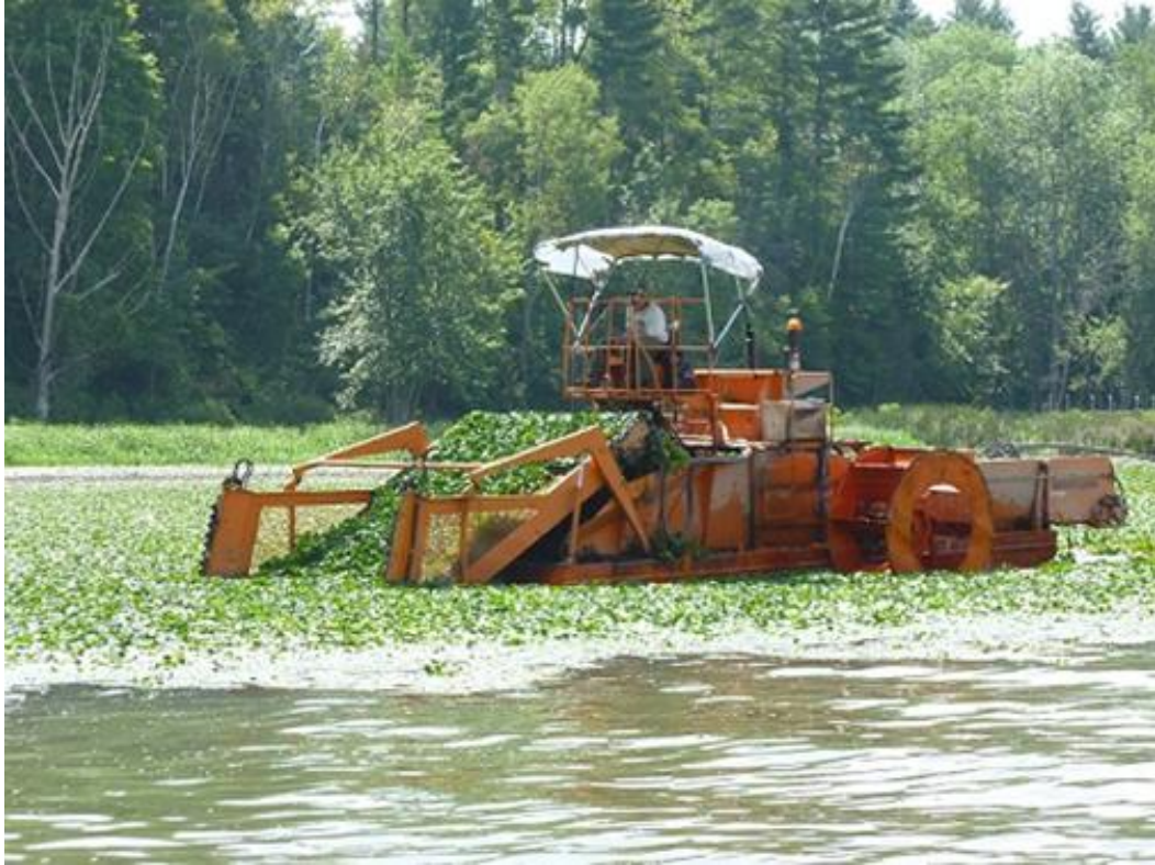
Figure 3-1. Aquatic invasive species mechanical harvester in a Vermont lake. Photo retrieved from https://dec.vermont.gov/watershed/lakes-ponds/aquatic-invasives/control .
