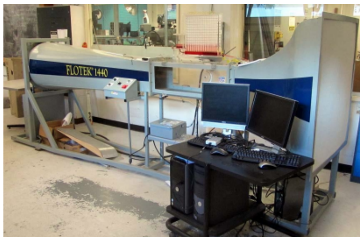
Figure 17: Flotek 1440 Wind Tunnel 18
