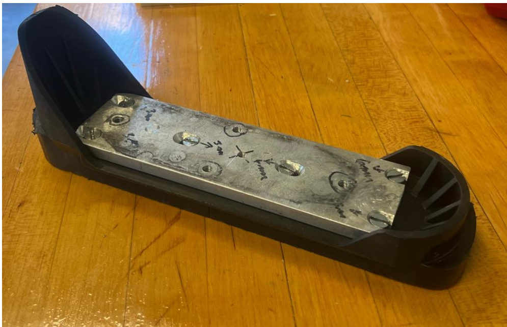
Figure 7: Test sole that is used as a representative of ISO 5355 alpine boot soles during alpine binding release testing
