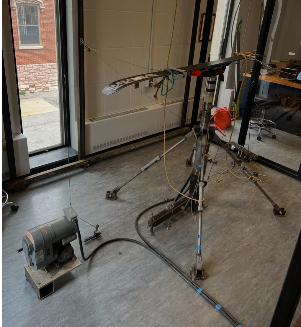
Figure 3: University of Vermont 504 Ski Binding Release Tester in the Ski Safety Test Laboratory consisting of two motors, a system of cables, and load cell.
