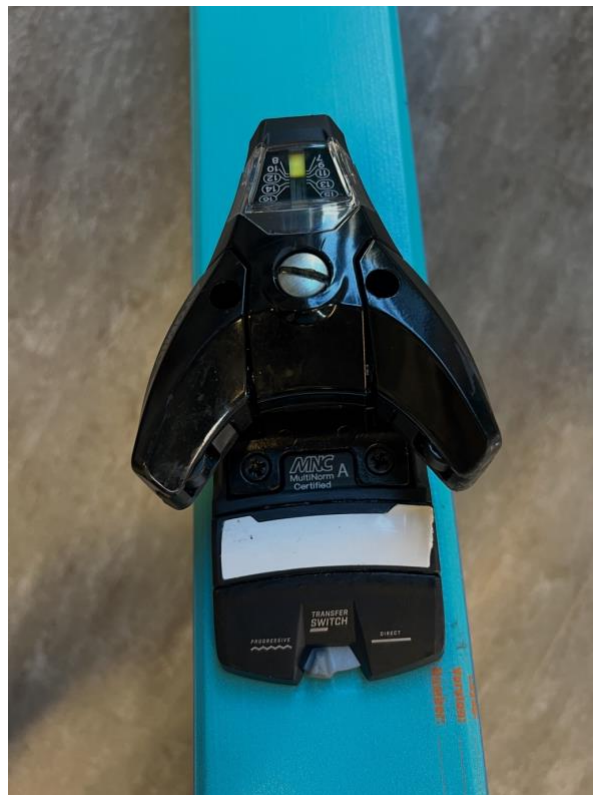
Figure 12: Multi-Norm ski binding, as denoted by “MNC” in the toe piece, used in multi-norm binding testing
