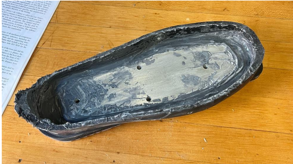
Figure 13: GripWalk sole after being cut and removed from boot housing and set with reinforcement plate and steel-reinforced epoxy. Holes drilled with mate with boot mount.
