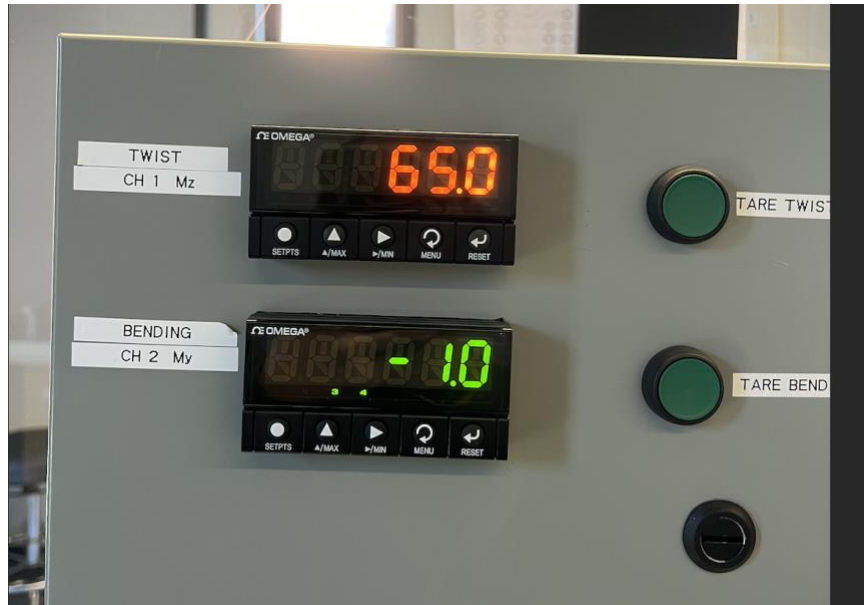
Figure 6: The digital readout system displays maximum torque during a release in the bending and twist directions.
