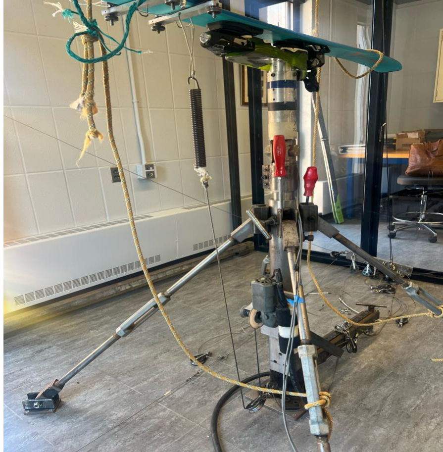
Figure 5: The 504 tester's smaller preload motor and spring system rotates around the center axis to provide front or rear preload.
