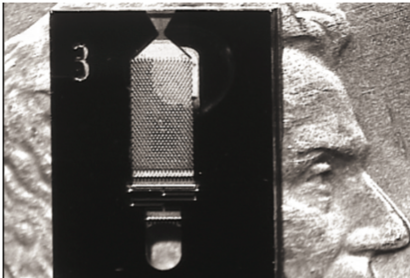
Figure 1.12: A digital photograph of the completed MEMS diamond pillar microthruster. A top view is shown, with the inlet at the bottom and the nozzle at the top of the figure. To provide a reference length scale, a US penny is included in the background. Reproduced from Hitt et al. [9]
