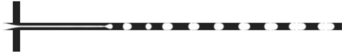
Figure 3.8: Sample surface plot of the baseline simulation. The liquid is represented in black, and the gas is represented in white.
